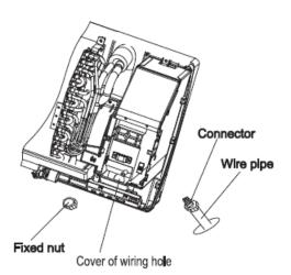
4. Wire pipe should be tightened by the fixed nut and the electric box should be fixed as shown in the above right figure and the below figure.
